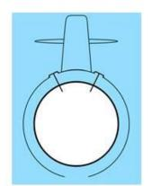
The water in the ballast tanks causes the submarine to submerge because the submarine becomes heavier than the water that would occupy that area.
