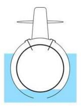
A submarine begins floating on the surface of the water. The inner circle represents the inner hull of the submarine. This hull on USS Razorback is 7/8" thick. The space between the inner hull and outer hull represents the ballast tanks.
