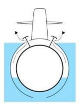
The ballast tanks are used to allow the submarine to stay on the surface or to submerge. The arrows at the top show that vents are opened by levers to allow the air to escape. Once the air pressure has changed the water enders the tanks.
