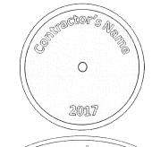
This round tag represents an inspection via a full 18" excavation and treatment with an approved paste. The tag shows CONTRACTOR's name and the actual year the work is performed.
