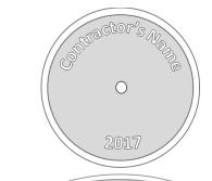
This round tag represents an inspection via a full 18" excavation and treatment with an approved paste. The tag shows CONTRACTOR's name and the actual year the work is performed.
