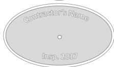
This oval tag is to be used whenever a sound and bore or partial excavate inspection takes place. The tag shows CONTRACTOR's name and the actual year the work is performed.
