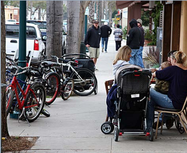
Sidewalks have three parts: the shy zone, the furniture zone and the walk/talk zone.
