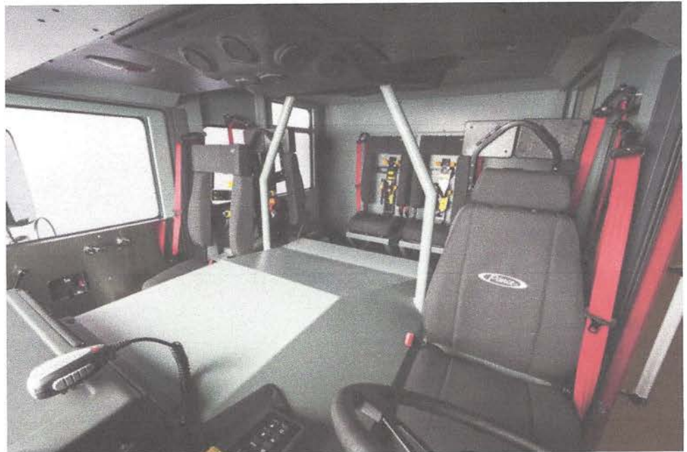
Smaller, lower engine tunnel maximizes driver and officer space while improving visibility across the cab All seats equipped with ReadyReach Seatbelts for easy usage in full gear
