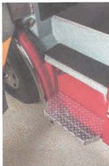
Low stair-style steps allow easier and safer exit/entry
